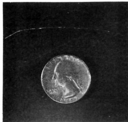
Figure 1. A fiber composed of the monopotassium salt of 5-(hexadecyloxy)isophthalic acid.
